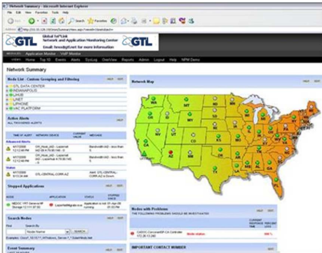
SNMP interface displays current network status and access to historical statistical data.
